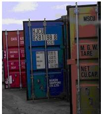
Look at the information on the rear doors. A container is generally marked with several items of information about the container's capacity: maximum gross weight, tare weight, net weight, and cubic capacity. Dry van trailers are rarely marked with information at this level of detail.
