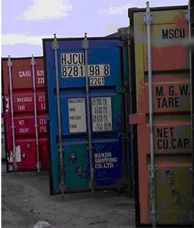
Look at the information on the rear doors. A container is generally marked with several items of information about the container's capacity: maximum gross weight, tare weight, net weight, and cubic capacity. Dry van trailers are rarely marked with information at this level of detail.
