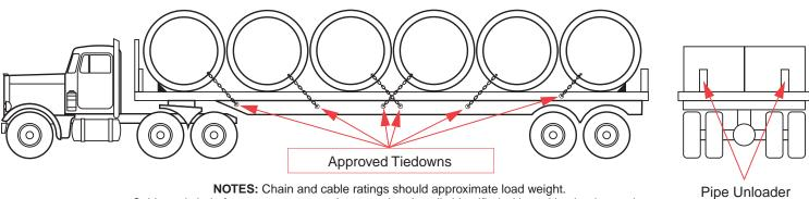
Cable and chain for securement must be tagged and easily identified with working load capacity.
