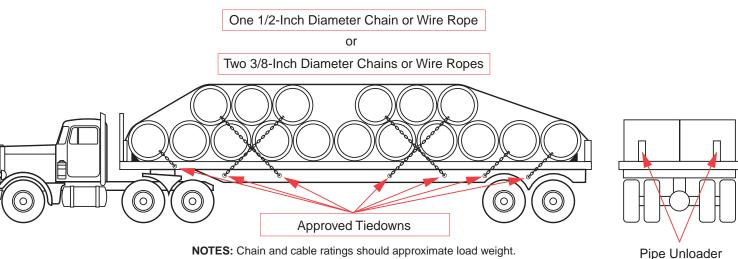
Cable and chain for securement must be tagged and easily identified with working load capacity.
