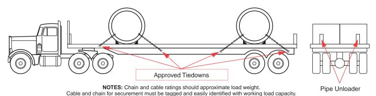
Transverse tiedowns shall run at an angle of not more than 45 degrees with the horizontal whenever practicable.
